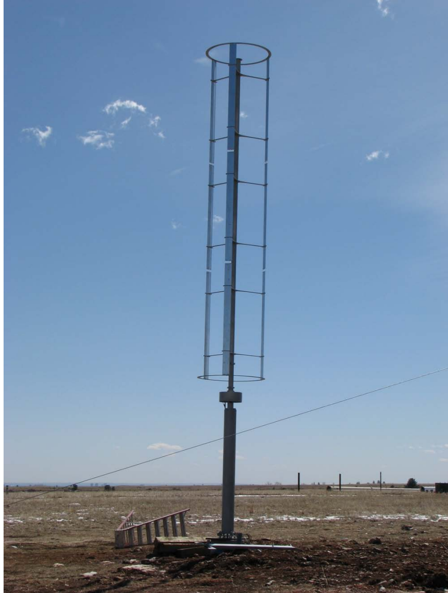
Figure 3. Mariah Power Windspire 1-kW test turbine at the NWTC
